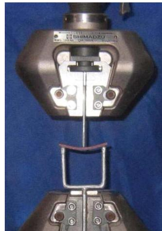
Fig 4: 3-point loading test in UTM
