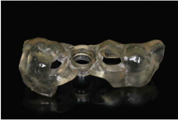
Figure 5: Printing of surgical template by using Formlabs Form 2 Stereolithographic 3D Printer
